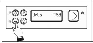
Press the pump-out button was and the display shows "UnLo" and the duration.
