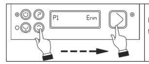
Press and hold it down to select the extra rinse function then press to confirm the program start.
