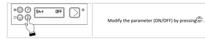
Set at "on" to start the cycle when the door is closed.
