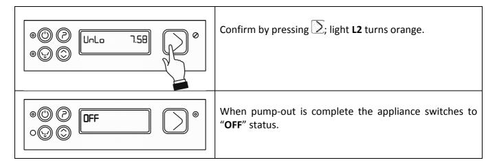
After a total pump-out the filters should be cleaned as described above.
