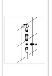
The **dynamic** water supply **pressure must** be between **1 and 6 bar**; if it is higher, installation of a pressure reducer is necessary.
