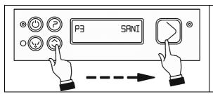
Press  $\circledcirc$  to select the sanitisation function then  $\widecheck{\ \ }$  to confirm the program start.
